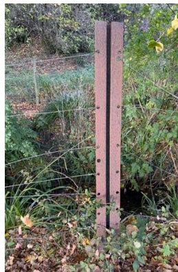
Short sections of iron rail, of the 'bridge rail' section devised by Brunel to match the iron-working technology then available, rather than the familiar 'bull head' section in current use. These were probably cast in the late 1830s, and incorporated into boundary fences after the original broad gauge was replaced by standard gauge in 1892
